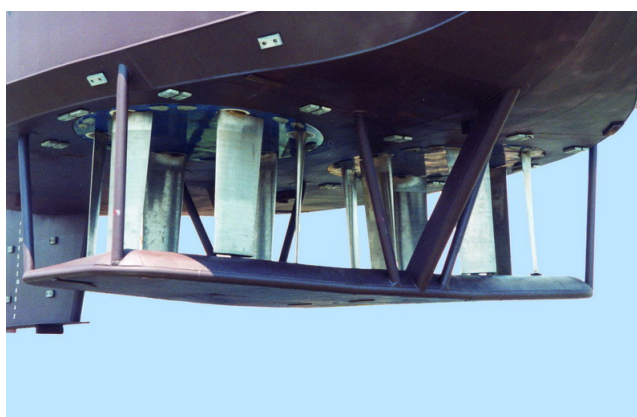
Figure 1.5: Twin Voith Schneider propeller with thrust plate on a tug's hull in dry-dock. [41]
